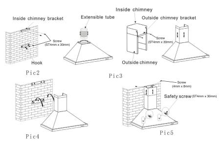
Warning: Failure to install the screws or fixing device in accordance with these instructions may result in electrical hazards.
