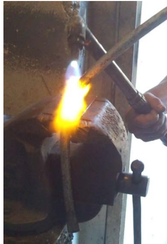
Figure 6-18: Heat bending of the water pipe with a torch
