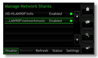
**Note:** Naming the Network Share must be done via the connected computer operating system. Network Shares are only enabled automatically if their name contains the words "music", "MP3" or "Content".
