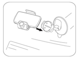
• In order to prevent the device from moving while driving, lock the mount in place using the included Allen wrench. Conversely, if you feel that the MINIKIT *Smart*'s magnets and its mount are inverted (repulsion rather than attraction), use the Allen wrench to unlock the mount's position and pivot its end.
