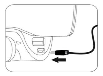
• The LED located next to the mini-USB port turns on to indicate that the battery is being charged. The LED turns off once the Parrot MINIKIT *Smart* is fully charged. It takes around 2 hours to charge the Parrot MINIKIT *Smart*.
