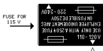
Figure 3.2. Fuse holder, here set at 115 V mains supply.
