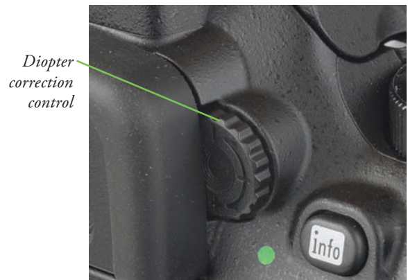
Figure 1.8 Viewfinder diopter correction from -1.7 to +0.5 can be dialed in.
