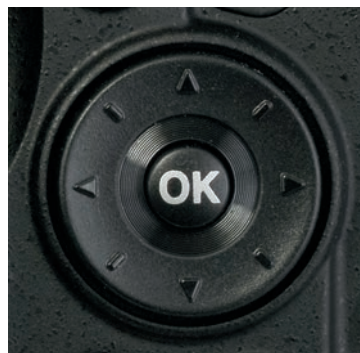
Figure 1.2 The multi selector pad has four directional positions for navigating up/down/left/right, and a center button to confirm your selection.
