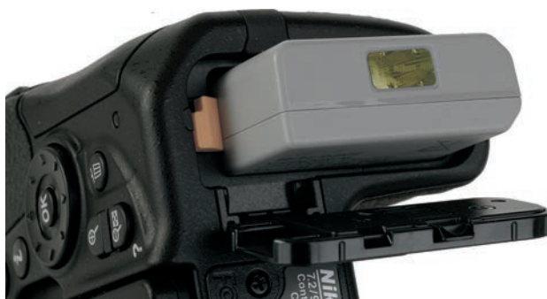
Figure 1.5 Insert the battery in the camera; it only fits one way.
