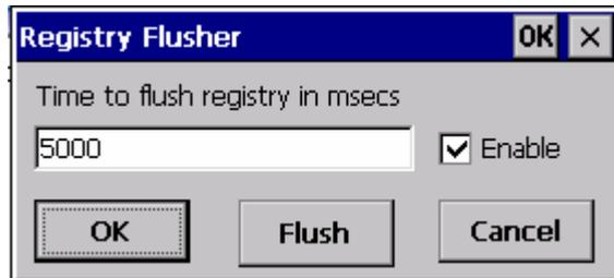
**Automatically:** Set time in milliseconds and check the enable box. The system will then save the persistent registry automatically.
