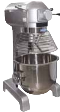
M1254 Planetary-mixer 20 Liter stainless steel bowl whip flat beater hook motor (HP): 1/2 480 x 410 x 760 mm Speed (RPM): 1) 110 2) 207 3) 371 Weight machine: 98 kg
