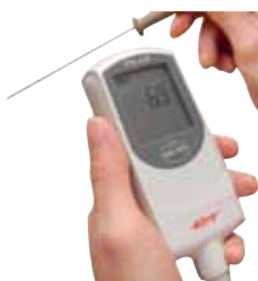
S5201 with heat-resistant (up to 220° C) power cord, HACCP approved and calibrated
