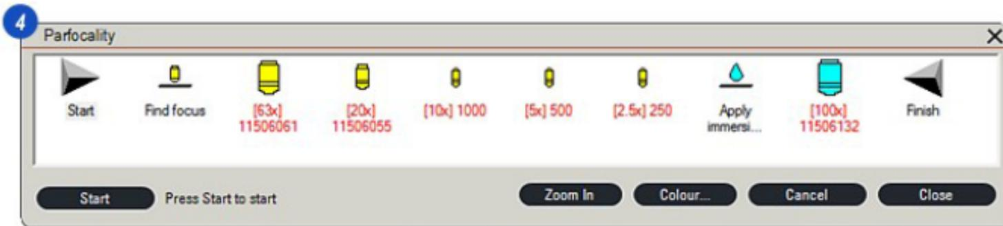
The selected objective blinks if you are changing the mode from *DRY* to *IMMersion* and vice versa. The stage is lowered and you have to confirm the change of mode with an additional mouse-click.
