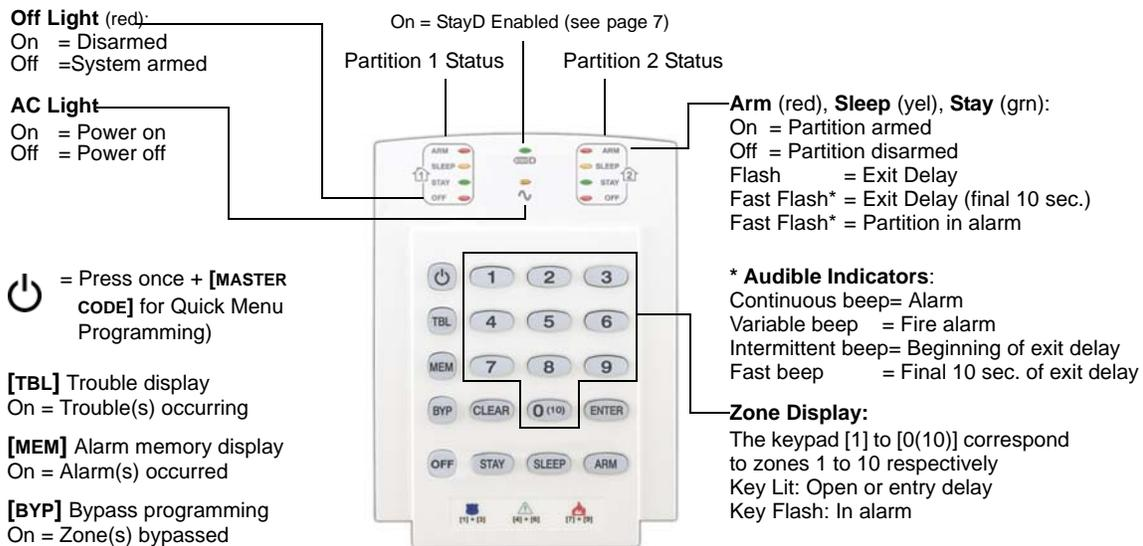
Figure 2: MG32LED —32-zone Hardwired LED Keypad
