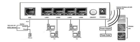
Notes: Without the splitter and certain situation, transient noise from telephone can interfere with the operation of the Router, and the Router may introduce noise to the telephone line. To prevent this from occuring, a small external splitter must be connected to each telephone.
