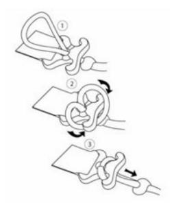
Important: Loop end of rope MUST pass through hole of the quick-connect prior to wrapping loop around hooks. Inspect condition of molded tow point prior to each use. Do not use if it shows signs of damage, cracking or breaking.
