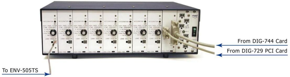
Figure 11 - ENV-505TS Load Cell Amplifier
