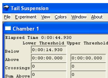
The **Elapsed Time** is how long the experimental session has been running. The **Below**, and **Above** refer to the amount of time spent below and above each Threshold for the current Block (see **Number of Blocks** and **Block Time** sections of this manual). **Crossings** represents the number of times the plot crossed above and then below Lower Threshold or Upper Threshold for the current Block. **Sum Above** is the total cumulative
