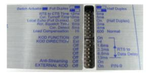
Align the pins of the KOD with the mating headers on the main board and plug it on. Secure it with two #4 screws and lock washers.
