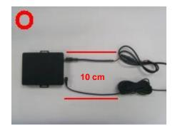
6. Connect one end of the power cable into DAB1002 and the accessory plug into car's accessory socket. There is a lock mechanism on the plug of Power Cable to DAB1002. Connect the DAB1002 before plugging in the accessory socket (see page 10).
