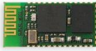
Figure 3.5 – Bluetooth Serial Converter UART Interface
