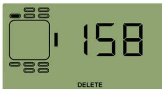
6. When finish programming these 3 digits, press S for 3 seconds to save with the screen flashes twice, beep buzzes twice. Then it will automatically switch to next tire position.
