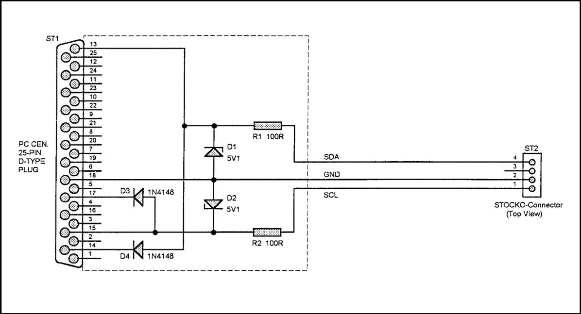
Figure 5 'Hardwareless' I<sup>2</sup>C Cable Configuration
