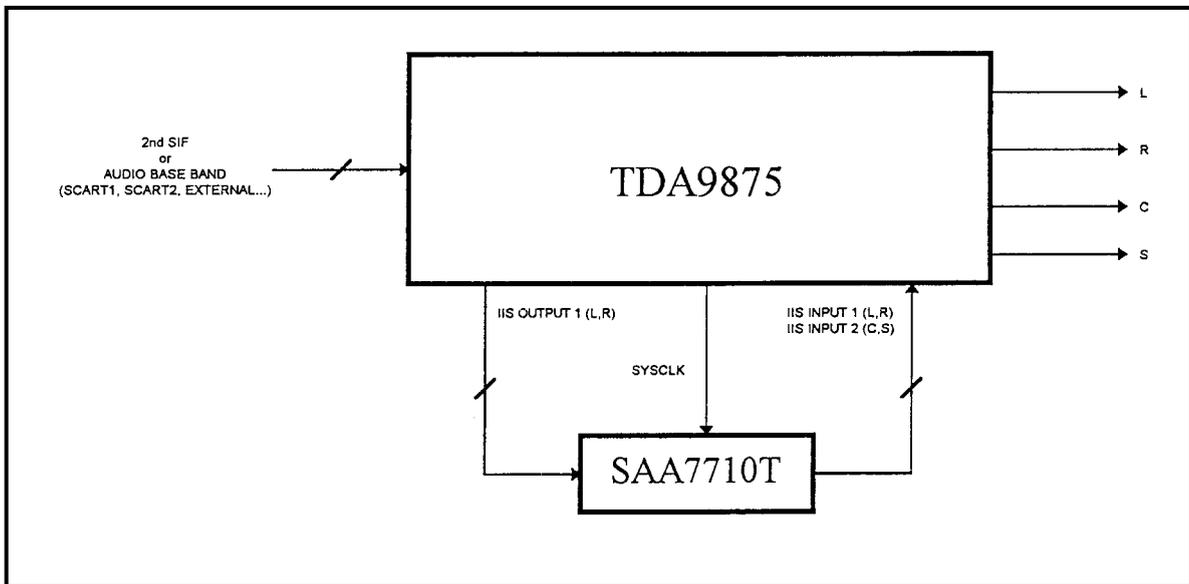
**Figure 3 Simplified Block Diagram for SAA7710T and TDA9875**
