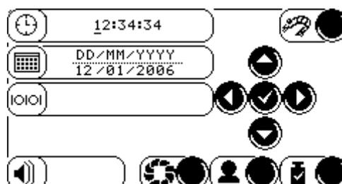
Using the arrows and the ok symbol all the parts of the screen can be changed
