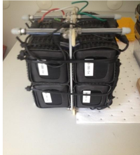
Figure 6 Four Batteries were configured for each canister
