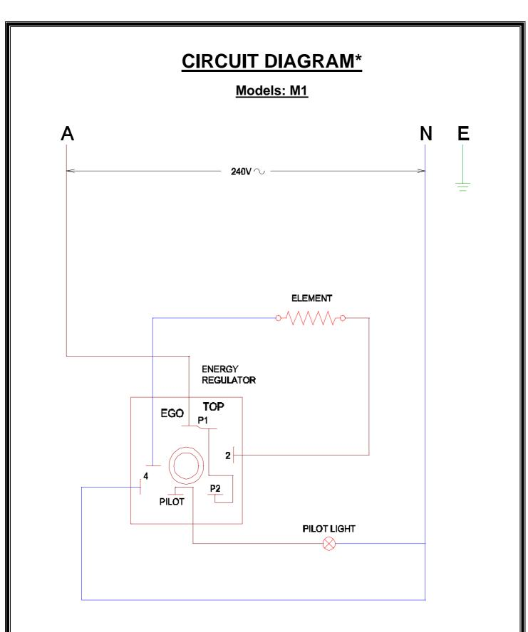
\* This circuit diagram has been provided for reference and to assist qualified service and repair agents only. Under no circumstances should person's not suitably qualified attempt repairs to any electrical equipment.
