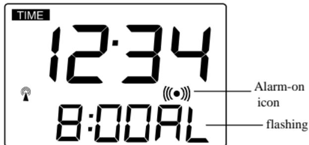
2. Press and release “AL/HOUR” to advance the hour, and “MODE/MIN” to advance the minute. The time will display in 24-hour format.
