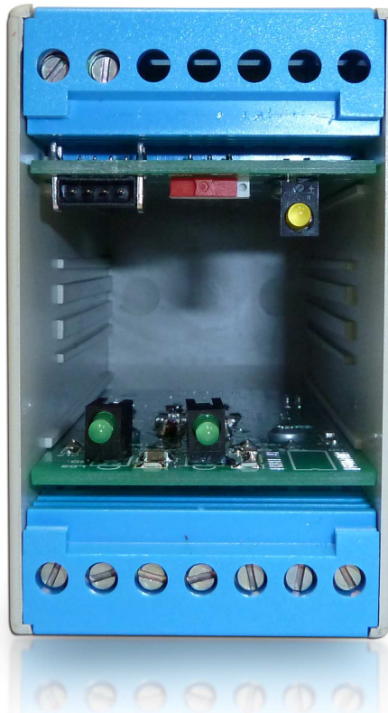
Photograph 2 Access to console port and programming switch
