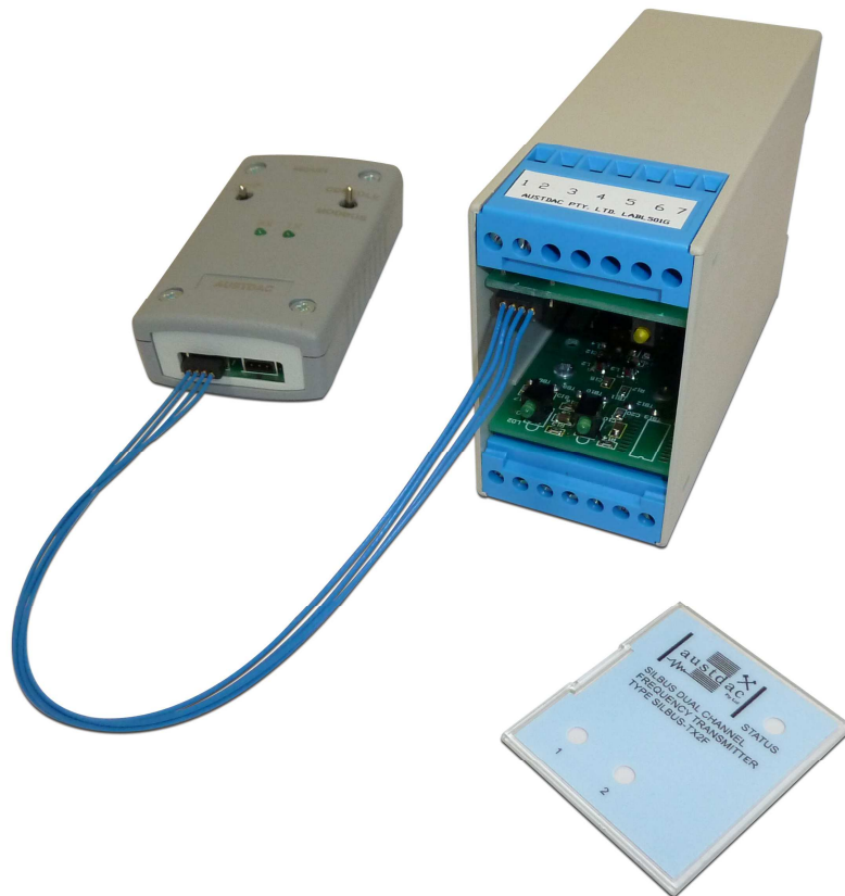
Photograph 4 SILBUS-TX2F console port connected to MEAN1 interface
