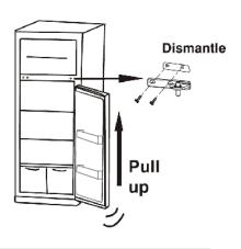
Remove the screws from the middle hinge. Lift the refrigerator door up and away from the appliance.
