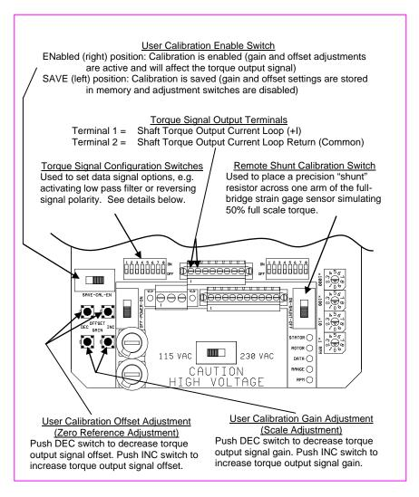
Figure 3 - Torque Output Controls and Connections
