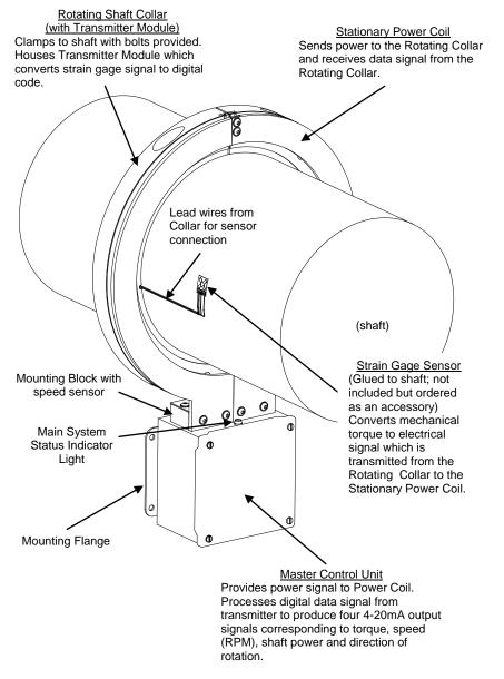
Figure 1 – Revolution System Components
