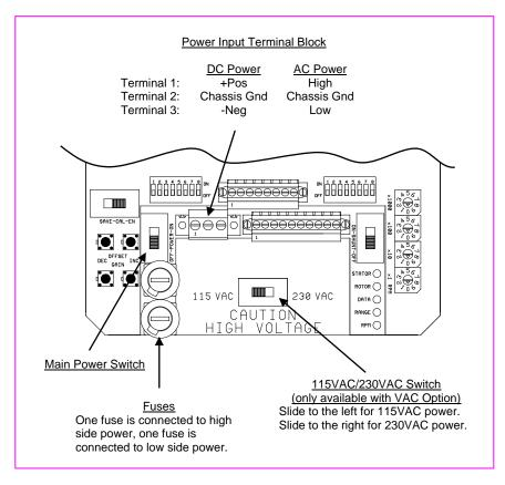
Figure 2 - Power Input Controls and Connections
