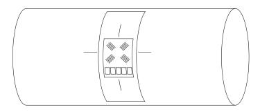
Positioning the Gage on the Shaft
