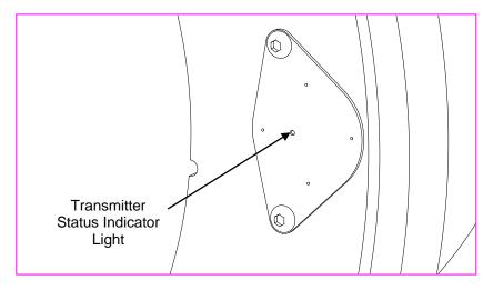
Figure: Transmitter Status Indicator Light
