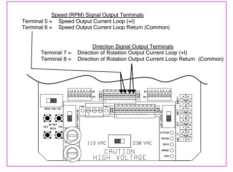
Figure 7 - Speed and Direction Output Connections
