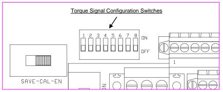
Figure 4 - Torque Signal Configuration Switches
