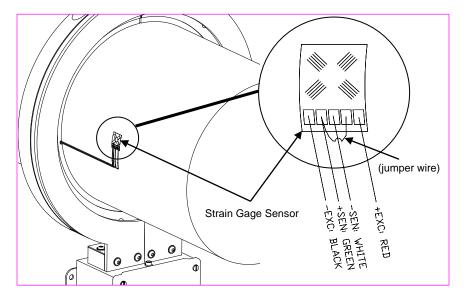
Figure 10 - Strain Gage Connections
