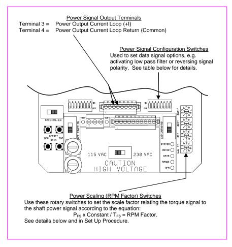
Figure 5 - Power Output Controls and Connections
