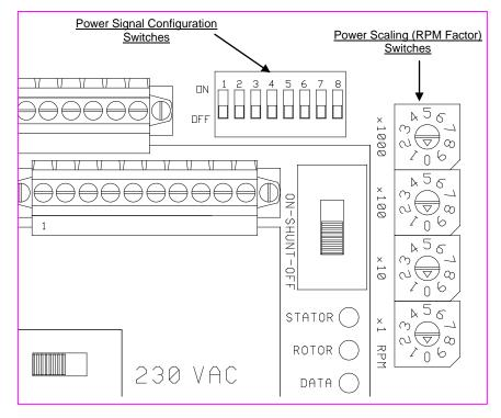
Figure 6 - Power Signal Scaling and Configuration Switches
