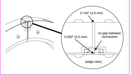
Figure 9 - Correct Collar Gap Spacing
