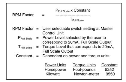
**Step 4: Set the RPM Factor rotary switches** in the Master Control Unit to the value calculated in Step 3. Turn system power OFF then ON to register new switch settings.
