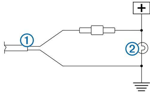
**NOTE:** Connecting the transmitter to an always-on 12-24 VDC source (such as a running lamp) instead of a reverse lamp requires you to manually switch power to the transmitter. The transmitter may drain your vehicle battery if it is left on.
