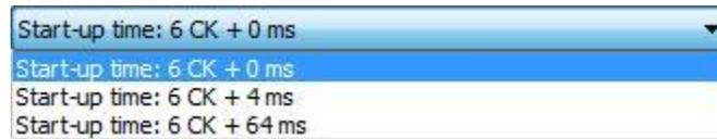
By default, chips that come from the factory have the **Internal 1 MHz clock with 6CK + 0ms Startup**.
