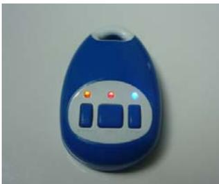
Switch on the unit outdoors. Three LEDs will light at the same time during the tracker starting.
