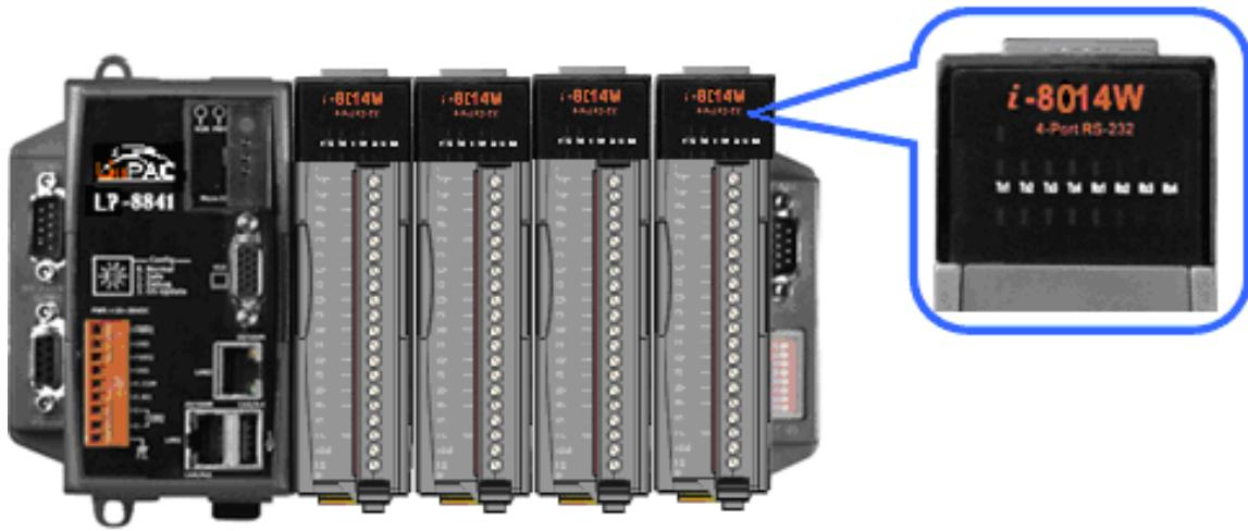
The I-8014W is a high performance analog input module. Up to 16-channel single-ended or 8-channel differential inputs can be connected to one module. It features 16-bit resolution, 250Ks/s sampling rates, and 4K-sample FIFO. It provides isolation protection of 2500 Vrms.
