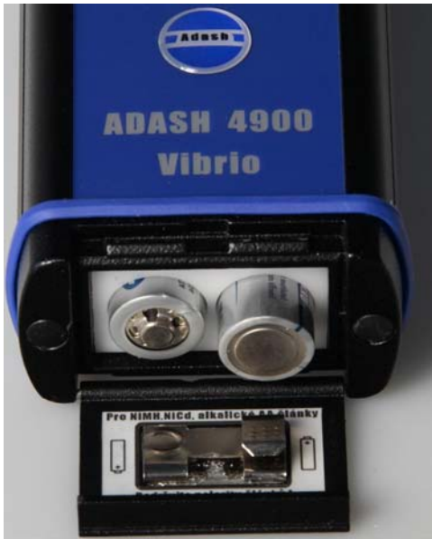
Fig. Placement of batteries
