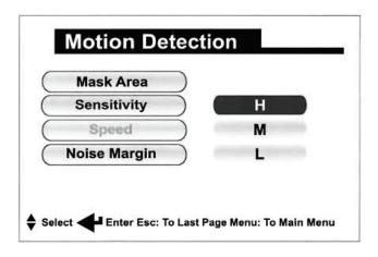
4) Press "OK " to enter "Noise Margin" to adjust the recording voice high / middle / low based on the environment voice.
