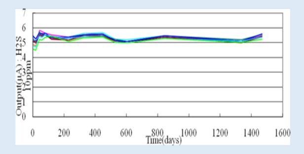
This data was generated in bench tests in a controlled clean environment. In service, in a real application, the long term stability will also be dependent on the environmental conditions of the application.
