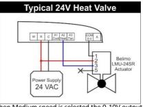
will be fixed at 6.6VDC. High speed is set to 10VDC
