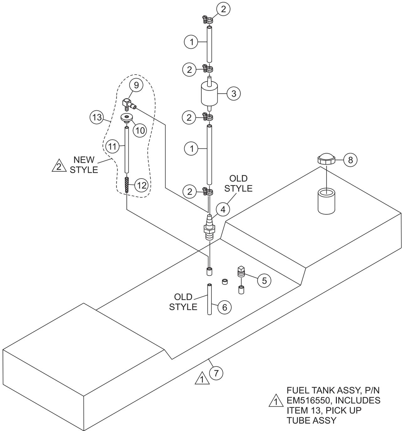
△ 1 FUEL TANK ASSY, P/N EM516550, INCLUDES ITEM 13, PICK UP TUBE ASSY
