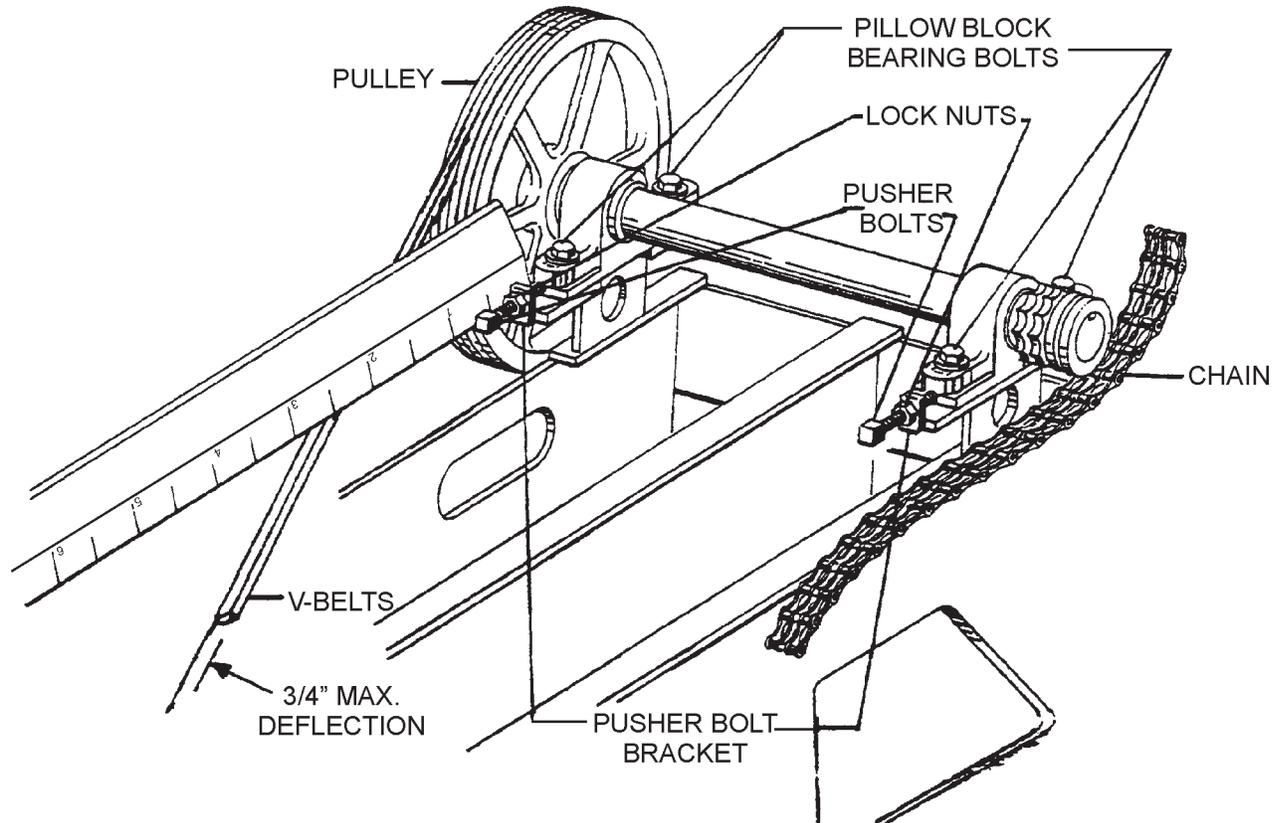
Figure 31. V-Belt and Drive Chain Adjustment
