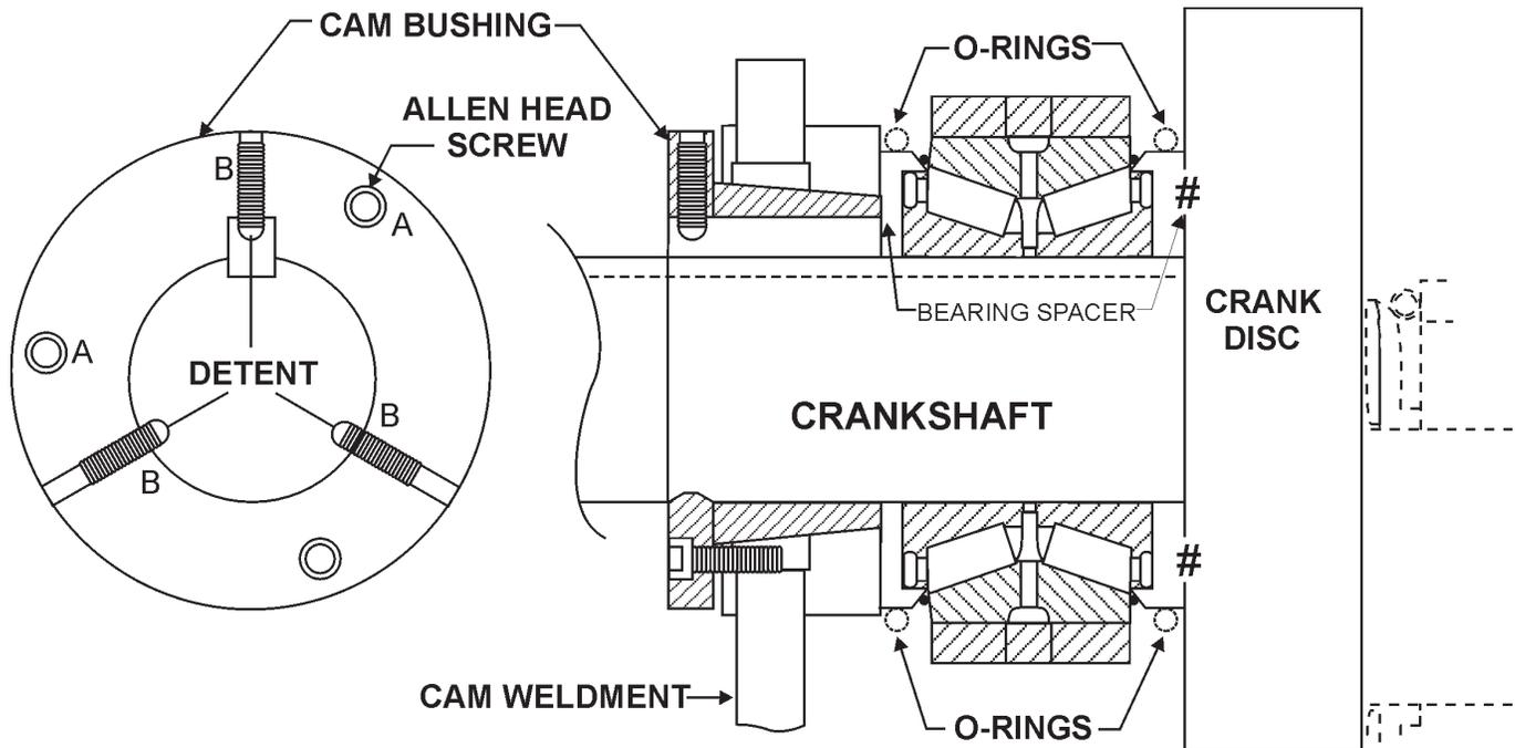
Figure 29. Bearing/Cam Bushing Installation
