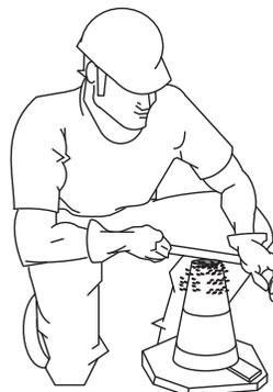
Figure 41-D. Slump Test (Removing Excess Concrete)
