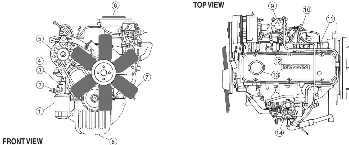
**Figure 6. Nissan Model A15 Basic Engine Components**
