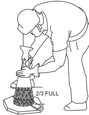
Figure 41-B. Slump Test (2/3 Full)
