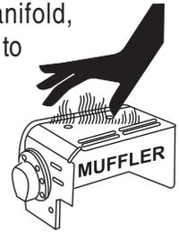
■ **High Temperatures** – Allow the engine to cool before adding fuel or performing service and maintenance functions. Contact with **hot!** components can cause serious burns.
