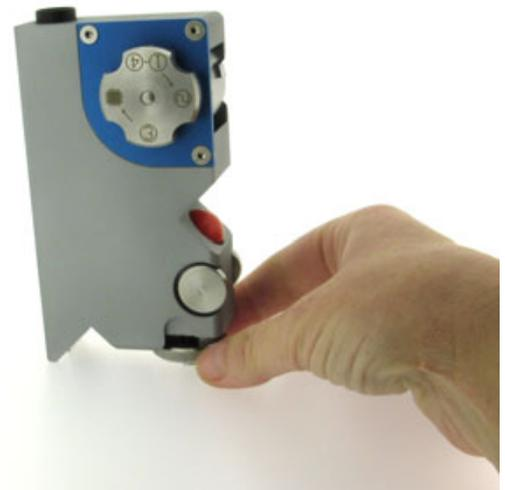
5. Read the graduation-scale and multiply the divisions with the D factor engraved on the SuperPIG.
