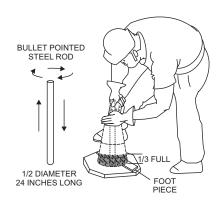
Figure 69-A. Slump Test (1/3 Full)
