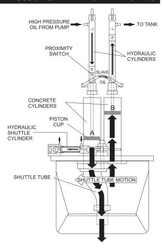
Figure 4. Pumping Cycle 2
