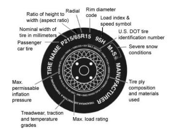
Figure 57. Standard Tire Sidewall Information
