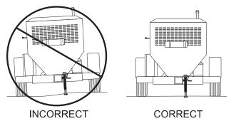
Figure 17. Rear Stabilizer Stand Deployment
