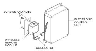
Figure 35. Installing Remote Control Module
