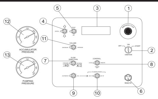
Figure 6. Pump Digital Control Panel Components
