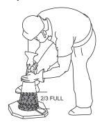
Figure 69-B. Slump Test (2/3 Full)
