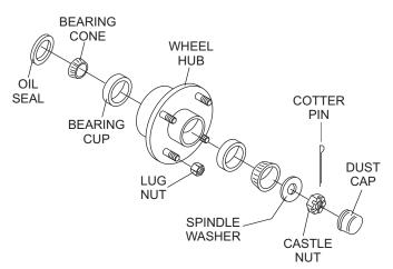
Figure 48. Wheel Hub Components Wheel Hub Adjustment
