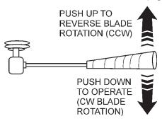
Figure 31. Hopper Remixer Control Lever
