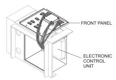
Figure 34. Pulling Out Control Panel
