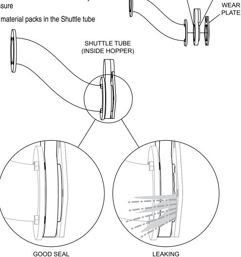
Figure A. Wear Plate and Cutting Ring
