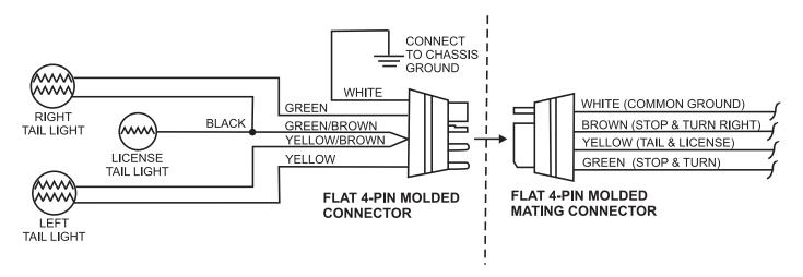
Figure 60. Trailer to Tow Vehicle Wiring Diagram
