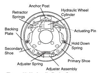
Figure 45. Hydraulic Brake Components
