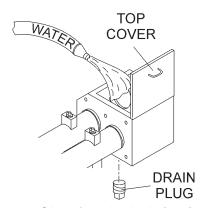
Figure 40. Cleaning the Lubrication Box
