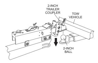
Figure 53. Ball Hitch Coupling Mechanism
