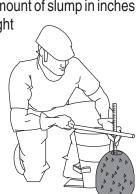
Figure 69-F. Slump Test (Measurement)
