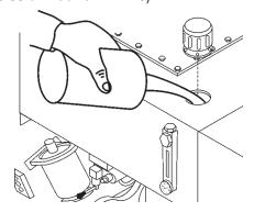
Figure 13. Hydraulic Oil Filler Hole
