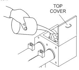
Figure 14. Filling the Lubrication Box
