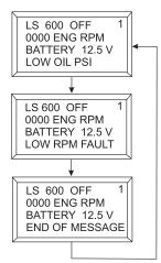
Figure 24. Primary Screen (Ignition Key ON)
