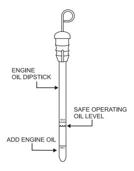
Figure 11. Engine Oil Level
