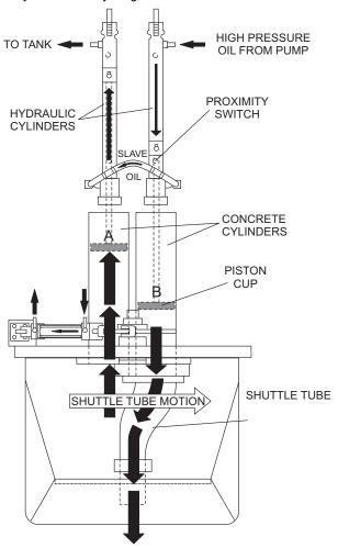
Figure 3. Pumping Cycle 1
