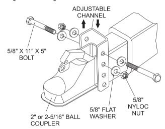
Figure 47. Adjustable Channel With Pintle Eye Coupler
