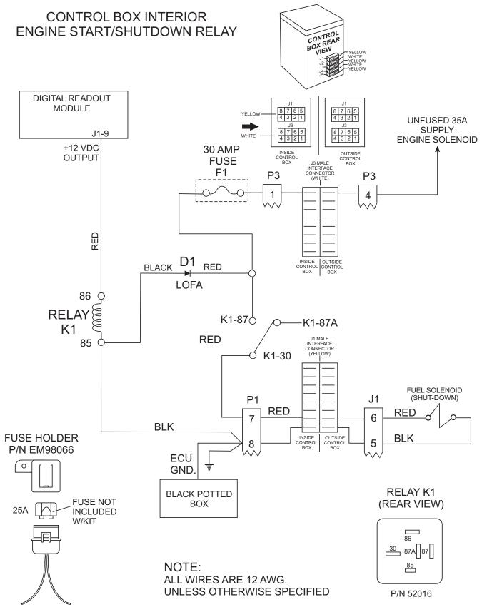
Figure 65. Engine Start/Shutdown Relay
