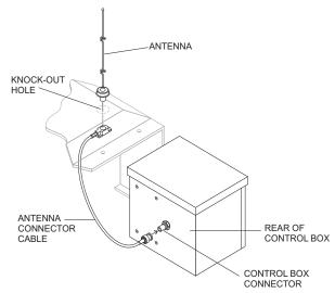
Figure 36. Antenna Installation
