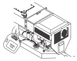
Figure 9. Adding Diesel Fuel
