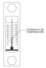
Figure 29. Hydraulic Oil Temperature Gauge
