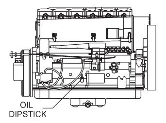
Figure 10. Engine Oil Dipstick
