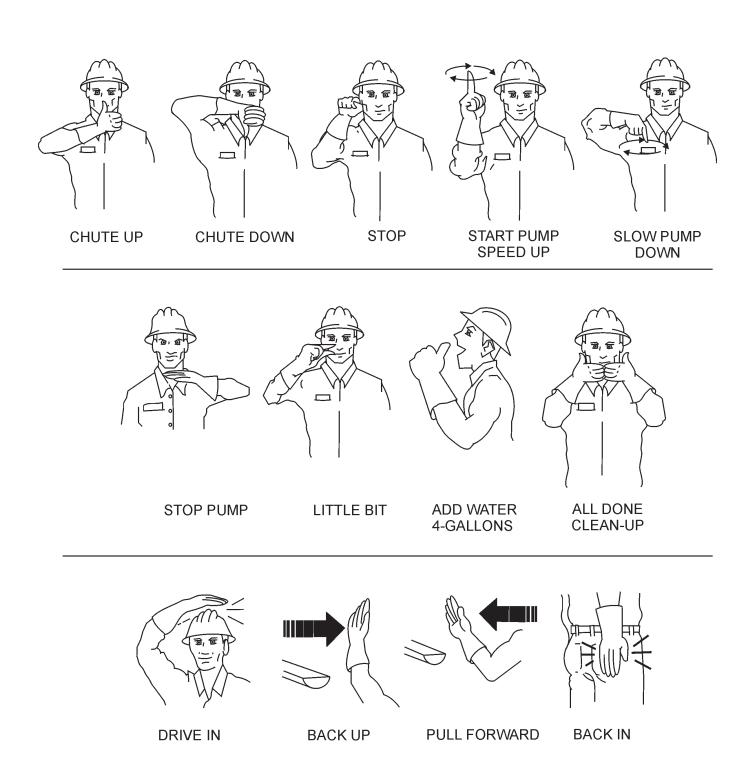
Figure 2. Operation Hand Signals
