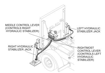
Figure 18. Control Levers for Hydraulic Rear Stabilizers
