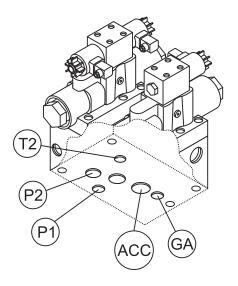
Figure 68. Manifold Block Ports
