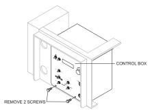
Figure 33. Removing Screws from Control Panel
