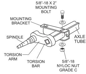
Figure 49. Torsion Suspension
