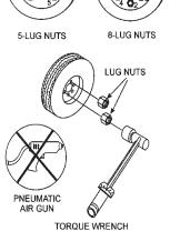
Figure 59. Wheel Lug Nuts Tightening Sequence
