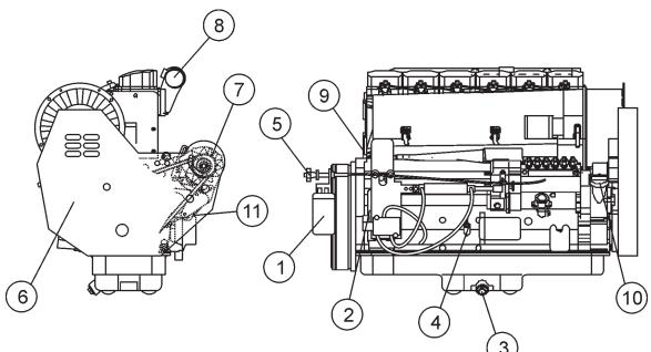
Figure 7. Deutz BF4L914 Diesel Engine Components
