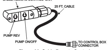
Figure 38. Cable Remote Control
