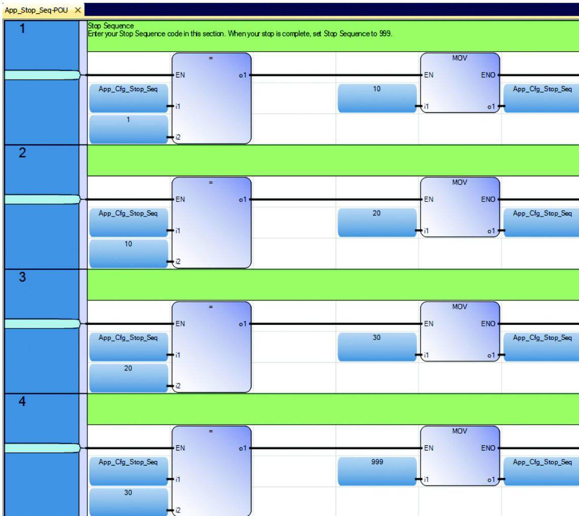
2. Modify rungs 1 and 2 in the App\_Stop\_Seq program to function like the example rungs 2 and 3, assuming you want the drive to stop when the machine stops.
