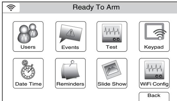
1. At the Master User screen select the WiFi Config icon. The system displays the WiFi options screen. The enabled recover mode will be displayed.
