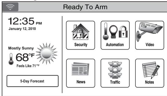
1. With the system in the disarmed or armed state, select the Video icon. The system advances to Cameras screen
