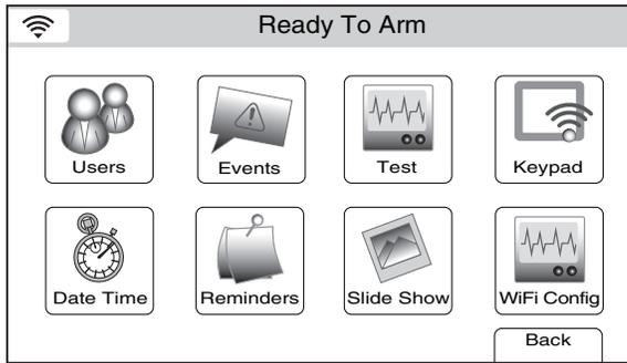
1. At the Master User screen select the Keypad icon. The system displays the WiFi devices screen.
