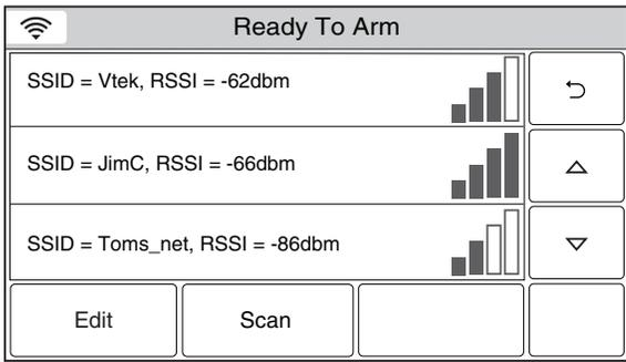
3. Select the desired Network and then select the "Edit" button. The network information is displayed. If a password is required, select the "Key" button and enter the password.
