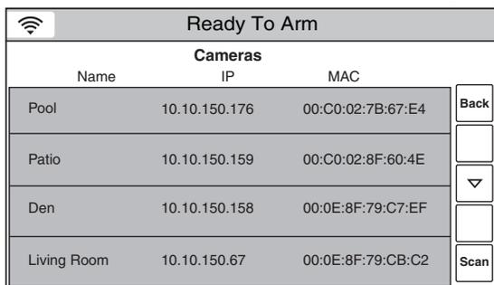
5. The selected camera(s) are highlighted. To edit the camera name go to step 6 OR to save the camera go to step 9.
