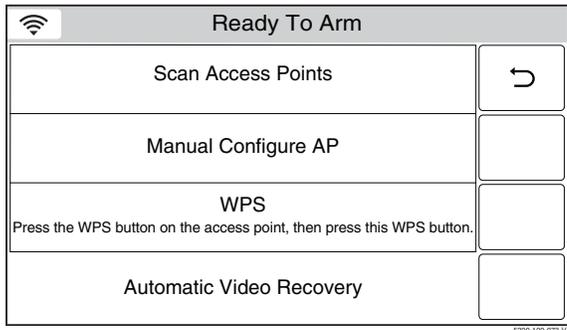
**Note:** For WPS operation, press the WPS button on the access point (router) first. Then press the WPS button on the control.
