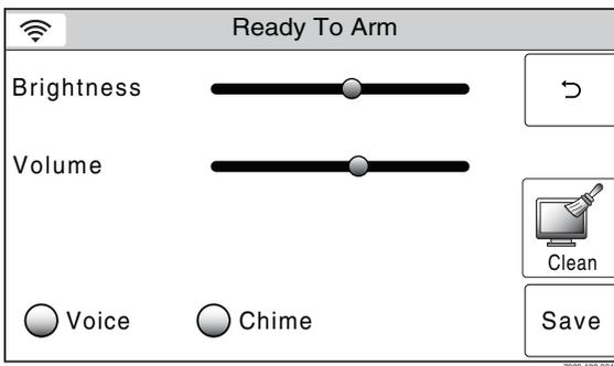
2. Increase or decrease the Display Brightness or the System Volume by using the sliding adjustment from left (decrease) to right (increase).
