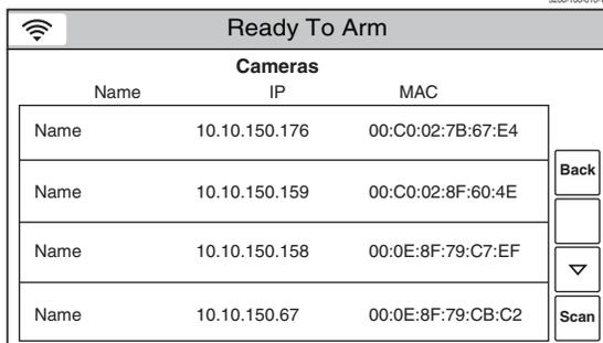
4. Select the desired camera(s) (up to four) from the list by "tapping" once. If applicable select the "▽" button to view additional pages of available cameras. Select the "△" button to return to the previous page of the list.
