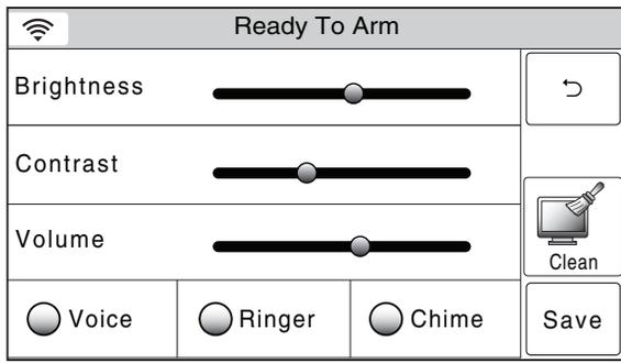
2. Select the “Clean” icon. The touch screen becomes inactive for a period of 15 seconds. A box displays “Please Use A Damp, Soft Cloth Touch Screen Will Be Disabled For 15 Seconds” and the time will count down.
