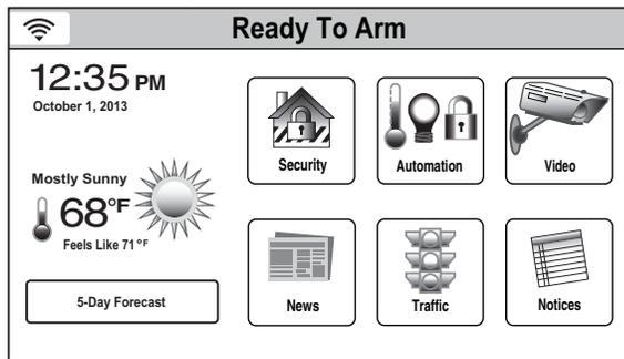
1. With the system in the disarmed state, select the “Automation” icon from the Home Screen. The system displays the first page of the Automation screen. Select the “▼” icon to advance to the second page of the Automation screen.
