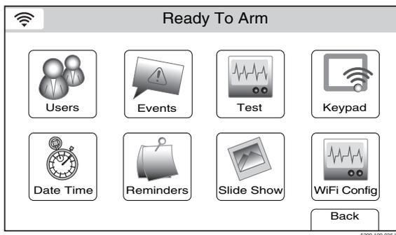
3. Select the “Test” icon. The system displays the Test screen.
