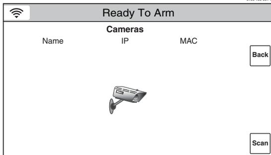
2. If no cameras have been discovered or if a list of discovered cameras is invalid, a Camera scan will start automatically.
