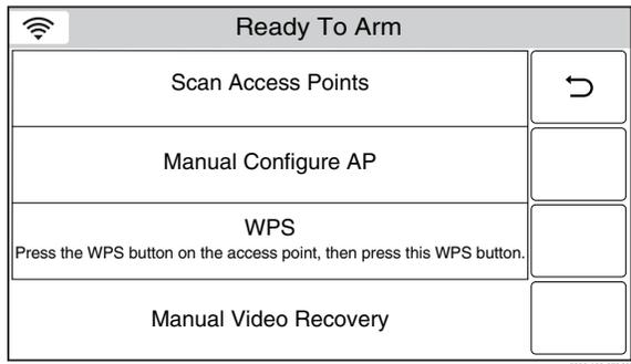
2. Selecting Automatic Video Recovery button will enable the manual feature or selecting the Manual Video Recovery button will enable the Automatic feature. The display toggles to display the selected mode and saves the entry.
