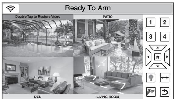
3. If Automatic Video Recovery is enabled, wait for the camera to automatically recover. If Manual Video Recovery is enabled, tap the video display two times to restore video.
