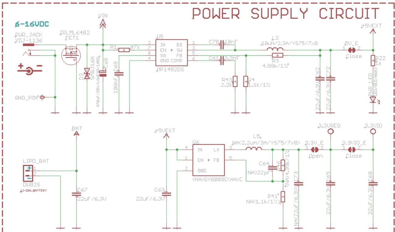
Note that the whole 3.3V part is not mounted (elements marked as NA) by default because we use the internal 3.3V DC-DC convertor in the iMX233. However, the internal DC-DC in the processor
