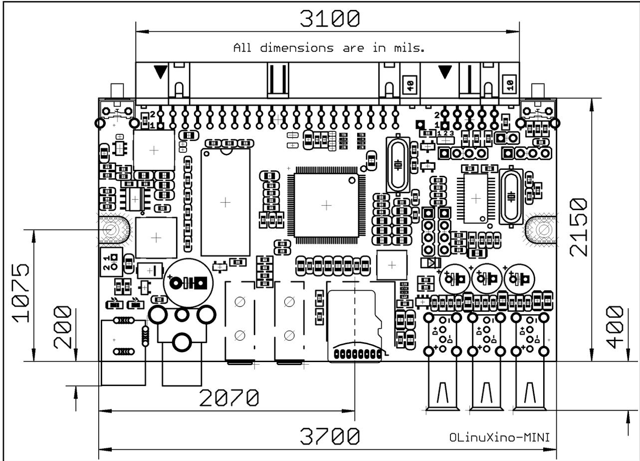
The three highest elements on the board in order from the tallest to the shortest are: capacitor C68 – 16.2mm (0.640") over the pcb; USB host connectors – 13.6mm (0.525"); composite connector – 12.0mm(0.464").
