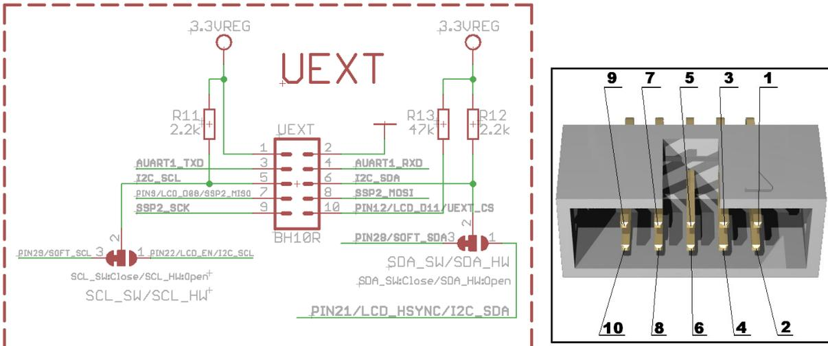
\*Note the two jumpers PIN29/SOFT\_SCL – PIN22/LCD\_EN/I2C\_SCL, and PIN28/SOFT\_SDA3 – PIN21/LCD\_HSYNC/I2C\_SDA which by default are set to a software SPI. They can be used to set the whole UEXT to a hardware SPI.
