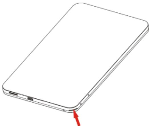
Locate and open the thumb catch on the lower right hand corner (viewed from the back)
