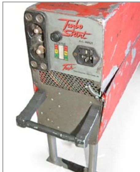
Figure 8.2.2 – Damaged Unit Misaligned Case with Bent Faceplate
