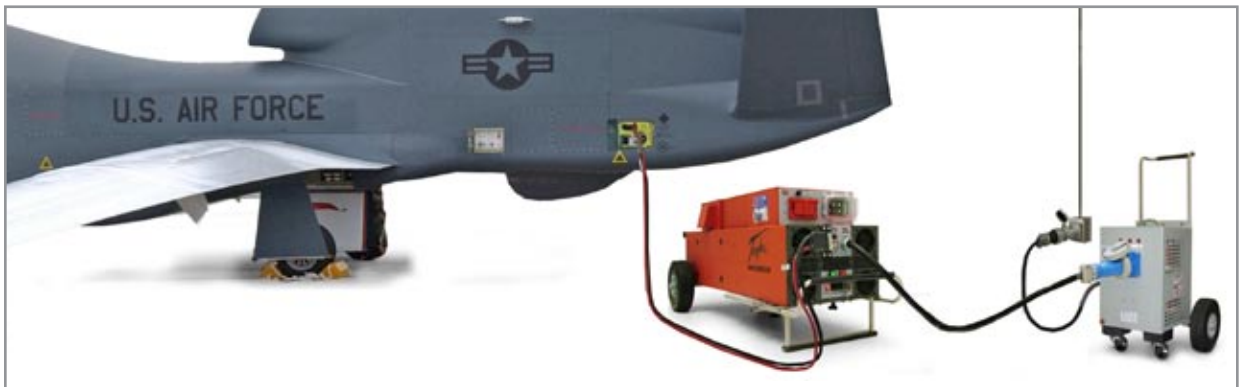
Figure 5.6.1 Connecting DC cable to aircraft and starting engine
