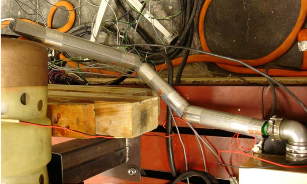
Figure 25: Exhaust as shield around power line.
