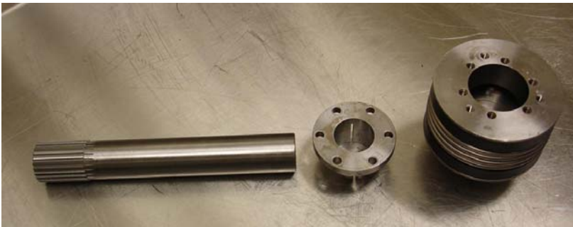
Figure 2: Input shaft and flexible coupling.
