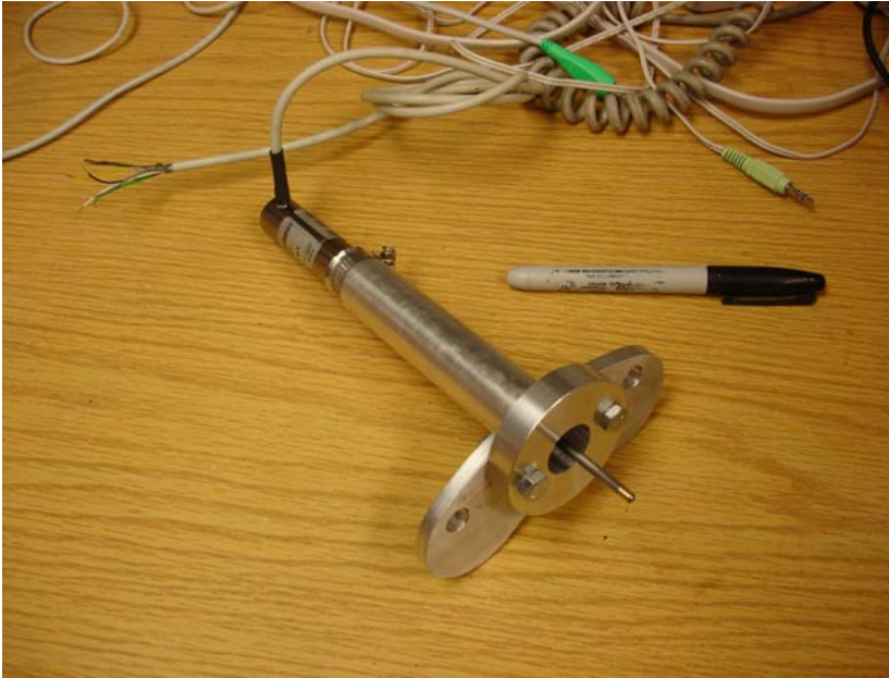
Figure 20: LVDT and mount
