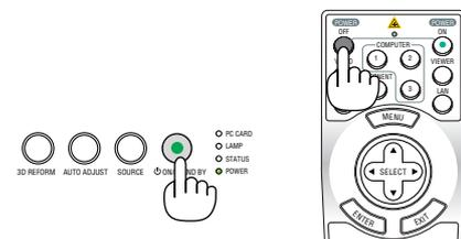
3. After making sure that the projector is in standby mode, turn off the **Main Power switch**. The power indicator will go out.
