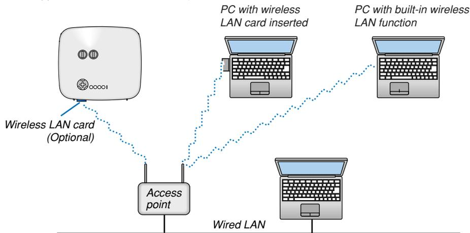
To make connection with a wired LAN via an access point, you need to select the Infrastructure mode.
