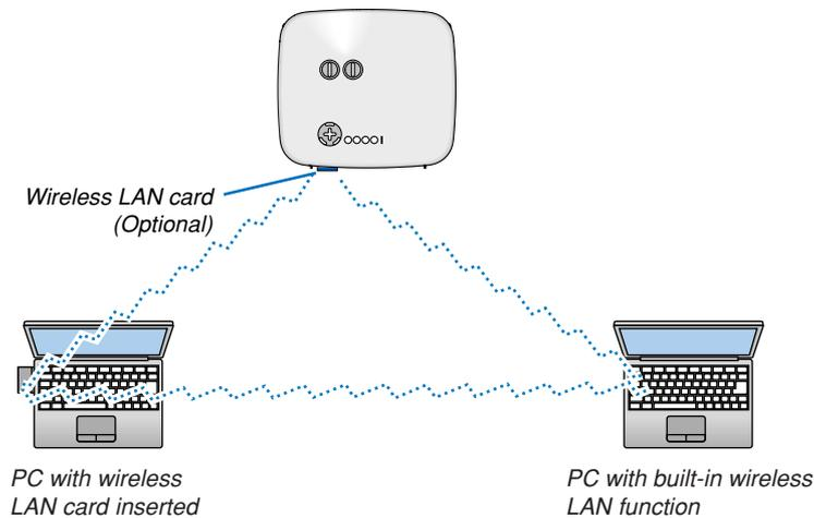
To enable direct communication (i.e., peer-to-peer) between personal computers and projectors, you need to select the 802.11 Ad Hoc mode.
