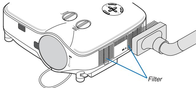
To reset the filter usage time, from the menu, select [Reset] → [Clear Filter Hours].
