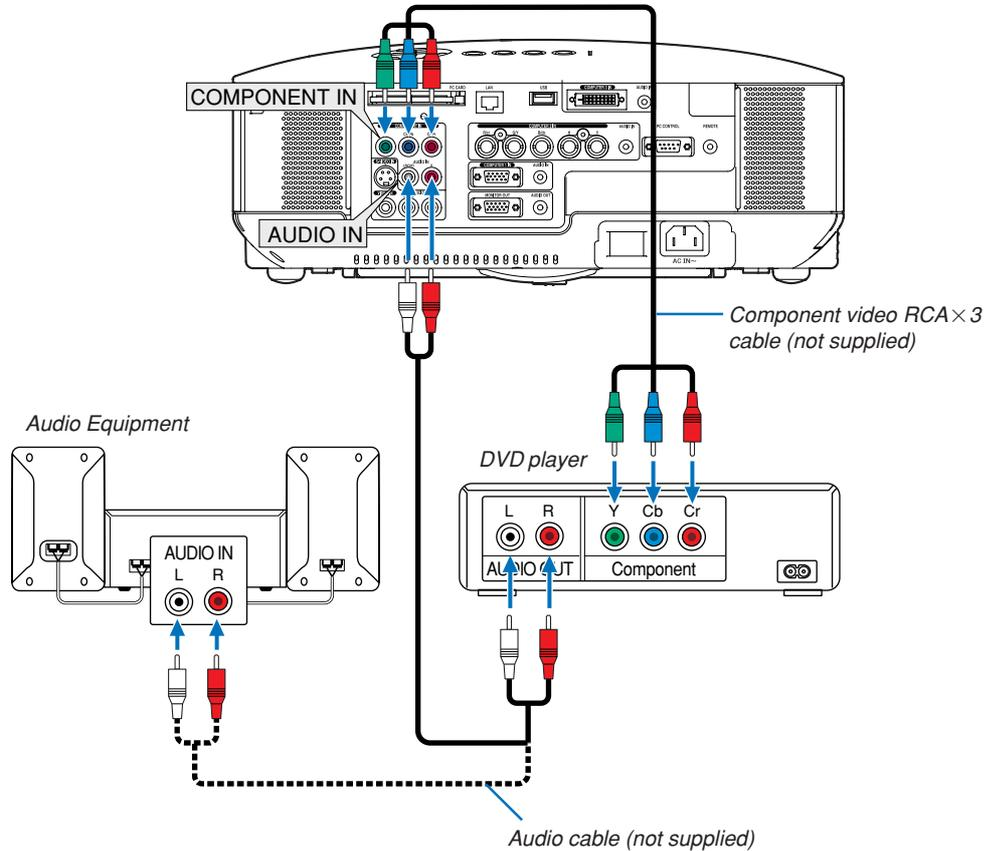
**TIP:** A component signal will be automatically displayed. If not, from the menu, select [Setup] → [Options] → [Signal Select] → [Computer 1 (or 2)] → [Component].
