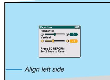
4. Press the SELECT ▲ button to select [Horizontal] and then use the SELECT ◀ or ▶ so that the top and bottom sides of the projected image are parallel.
