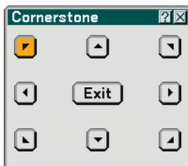
This option allows you to correct trapezoidal distortion. Selecting this item will display the Cornerstone adjustment screen. (→ page 41)
