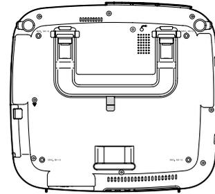
2. Pull up the carrying handle with the catch pressed down.
