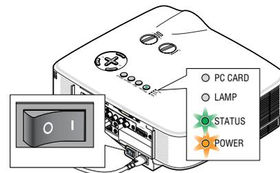
**3. After making sure that the projector is in standby mode, press the POWER (ON/STAND BY) or POWER (ON) button for a minimum of 2 seconds when the STATUS indicator goes off and the POWER indicator starts blinking.**
