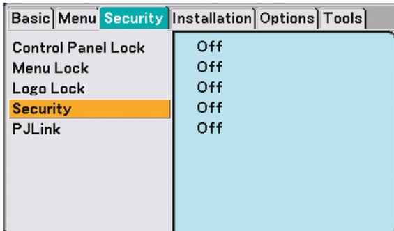
5. Press the **ENTER** button to display the Security screen.
