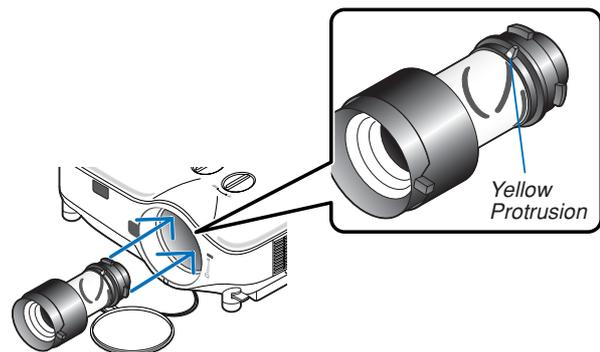
2. **Rotate the lens clockwise.**
