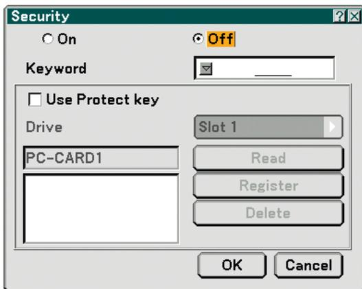
6. Press the **SELECT ▼** button once to highlight the Keyword entry box and press the **ENTER** button. The Software keyboard will be displayed.
