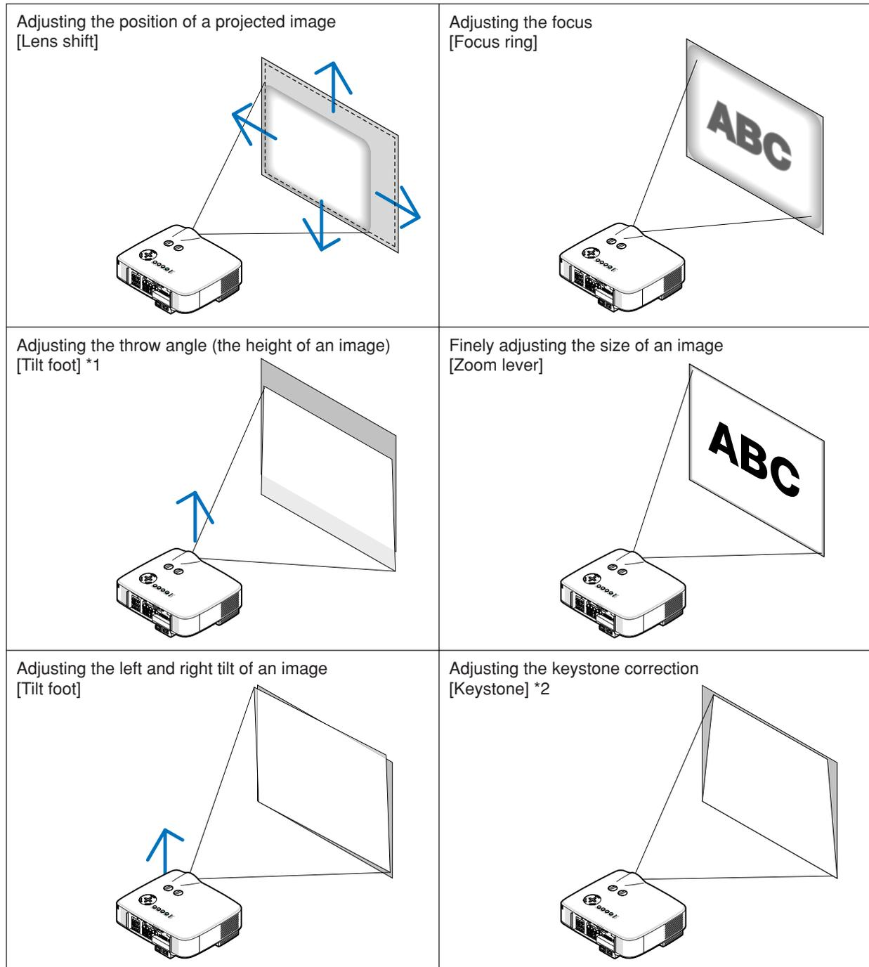
NOTE\*1: Adjust the throw angle (the height of an image) when the image position is higher than the lens shift adjustable range.
