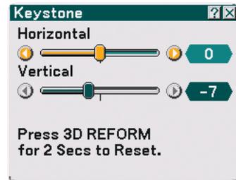
2. Press the SELECT ▼ button to select [Vertical] and then use the SELECT ◀ or ▶ so that the left and right sides of the projected image are parallel.
