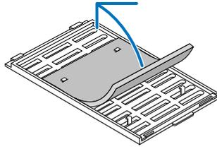
*The filter is attached self-adhesive tape. Peel off a release paper before use.*
