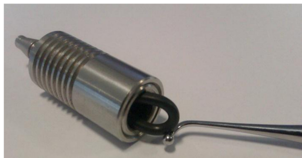
Figure 7: Inserting a new O-ring into the back-pressure adapter.
