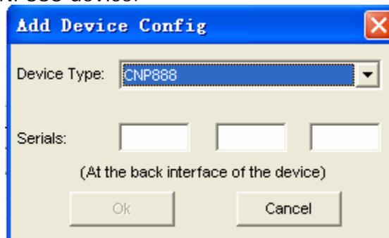
Enter the serial number of CNP888 device and select the correct device type (the serial number is labeled on the rear panel of the CNP888 device). Click "OK" to add the configuration.
