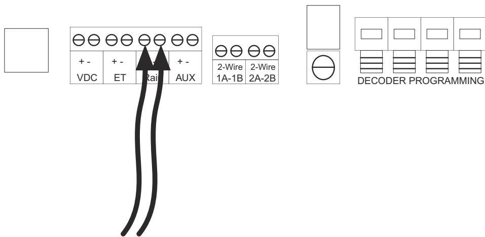
**Important!** Be aware of the polarity when you connect devices to the LTD: Connect plus to plus and minus to minus or you won't see the expected behavior from the connected devices.
