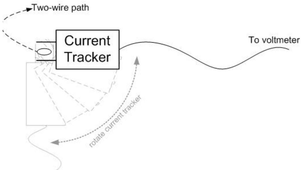
Ideally, you should rotate the current tracker around the individual wires inside the two-wire - do this if enough plastic is stripped off the two-wire.
