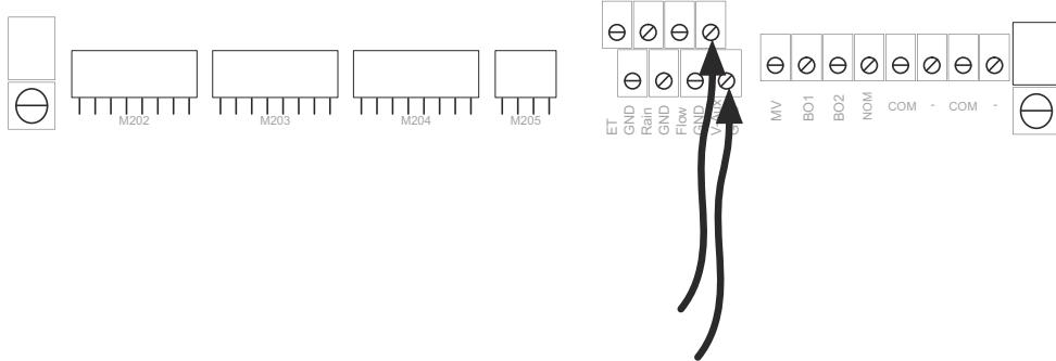
**Note:** An alarm is used instead of a Flow Sensor. Turn the dial to SENSOR SETUP and select N/O eller N/C.
