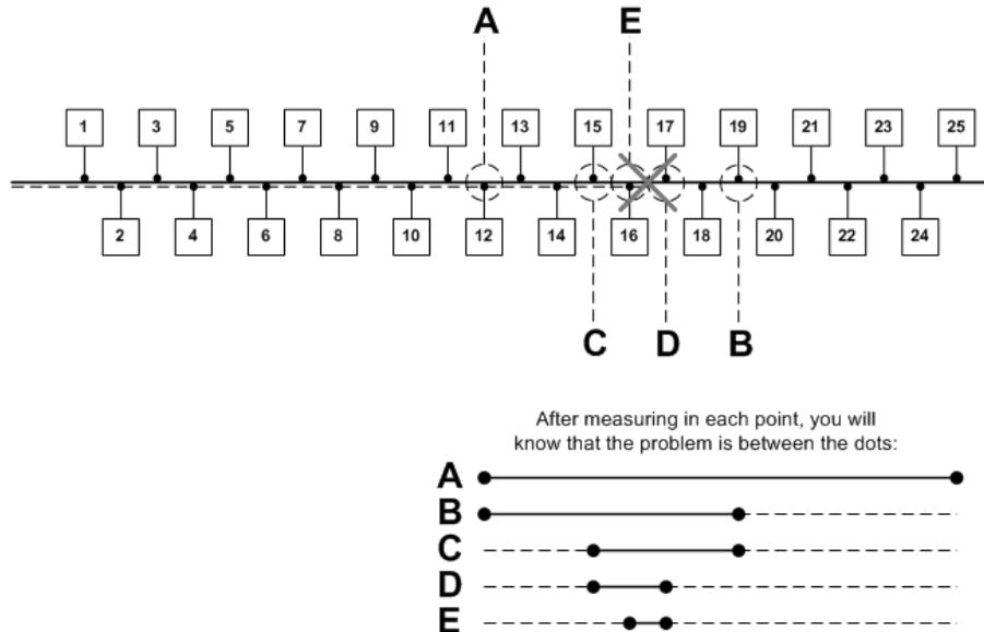
Looking at the graphic below we imagine that current is running at decoder 1 but no current is running at decoder 25. To start the binary search we measure in the middle, at point A:
