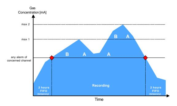
As soon as an alarm of the concerned channel is activated the measurement values which have been temporarily recorded in the past two hours are written to the memory card.
