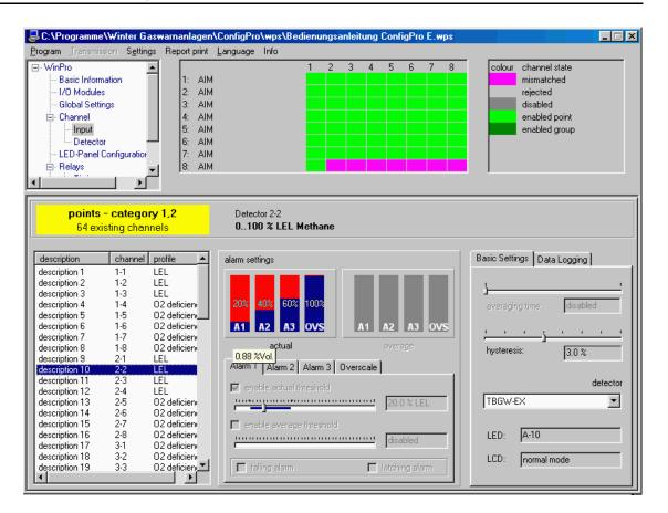
Under ,Input Settings' all alarm-related parameters can be accessed. By pushing the right mouse button it is possible to select the view. It is possible to show all measuring points, only activated measuring points or only configured measuring points. This filter also provides the view of measuring groups (see chapter 6.4.4 "measuring groups")
