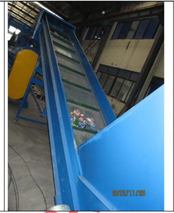
All the frame and support are made of carbon steel
