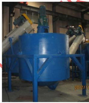
This device is connected with steam boiler. Steam is supplied into washing tank to heat water and flakes. Hot water makes dirt, label and glue water loosen from bottles. Meanwhile you need to add caustic soda and other cleaning chemicals into tank to clean bottle flakes.
