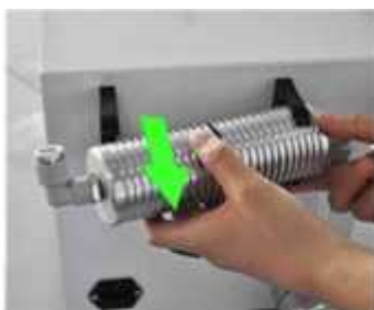
1. Remove the filter1
