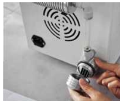
2. Take out the black filter cotton, clean the dust.
