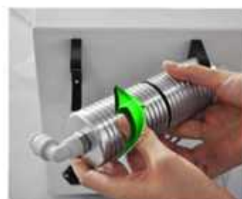
2. Take out the black filter cotton, clean the dust.
