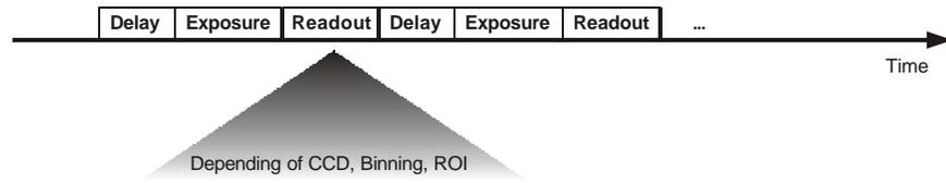
**Internal trigger "auto simultaneous"**
